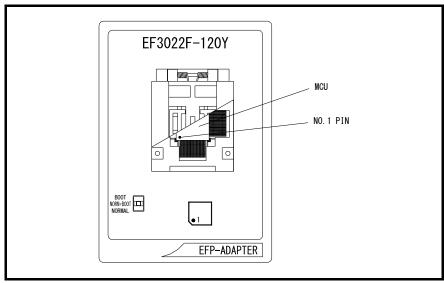
Figure 2.1: Pin Orientation of The socket
